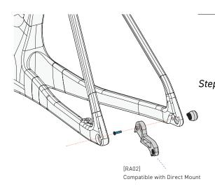
Step 9 We also have [RA02] direct mount hanger option, compatible with Shimano's direct mount rear derailleurs. During installation please refer to Shimano's instruction manual to remove the rear derailleur and its related components.
