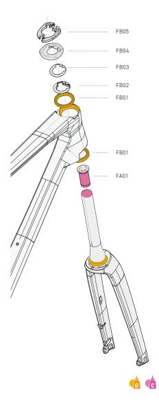
Step 3.1 Prepare the frame, fork, headset bearings, headset cap, headset washers, stem, and handlebar, and confirm the number of headset washers needed below the stem.
