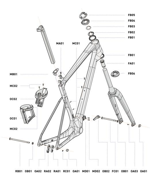
PA-AFO cables are wired completely internally, so assembly must be done with extra caution. We strongly recommend that you test assemble and complete your bike fitting prior to final bike assembly.
