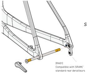
Step 9 PA-AFO comes with a [RA01] standard hanger compatible with SRAM and other standard rear derailleurs.
