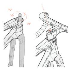
Step 3.2 Make sure that the fork, headset components, and stem fit together properly. Mark a line on the fork at the top surface of the stem, you'll be trimming the tube at 4.5mm below this line. This leaves just enough space for the headset cap (and includes the height of the fork plug expander).
