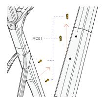
Step 11.1 Before installing, please unscrew the [MC01] bottle cage round stainless screws from the frame.
