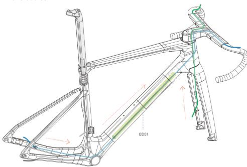
Step 5.4 Rear brake cable: Route the rear brake cable through the left chainstay, running through the bottom bracket and exiting through the top of the head tube. Cut a [OD01] foam cable sleeve to a similar length as the down tube, slide onto the cable, and adjust the sleeve's position to sit inside the down tube.
