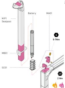
When placing the [MA01] seatpost clamp, tilt the bike 30 ~ 60 degrees or use tape to prevent the clamp from falling into the seat tube.
