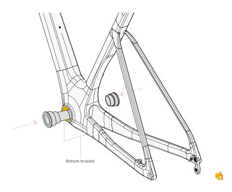
To avoid damaging the frame and bottom bracket, please use a bottom bracket bearing press when installing the bottom bracket. When using the bottom bearing bracket press, follow the press manufacturer's instruction manual.
